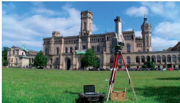
Figure 2: Nikon SLR camera and Riegl LMS Z360I scanner assembly
