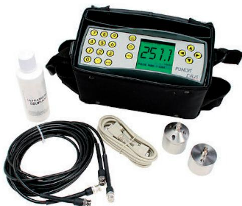
Figure 4: The Pundit Plus Ultrasonic system used
