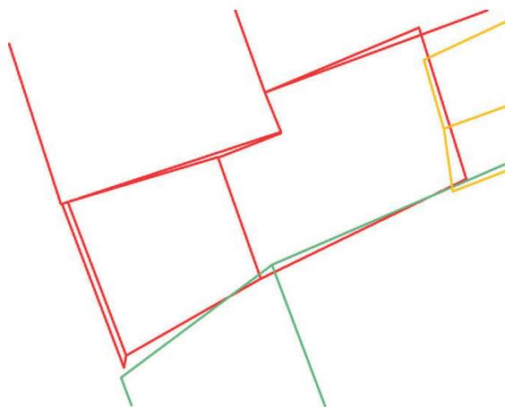
Figure 11: Interaction of three different roof skeletons in three different colours. One can see the parallelism errors between segments.
