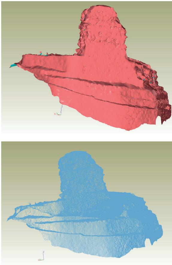
Figure 10: 3D mesh of the medieval tower
