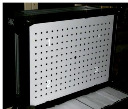
Figure 6: Calibration master for the common calibration
