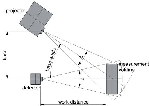
Figure 3: Measurement system setup
