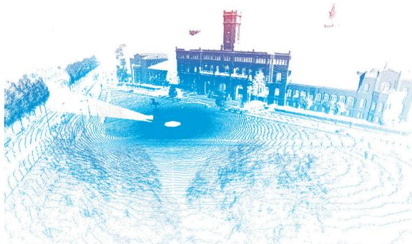
Figure 10: Terrestrial laserscan with color indicating height
