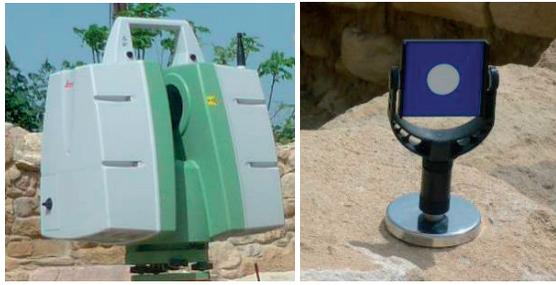
Figure 7: Leica ScanStation C10 (left) and the special targets (right)
