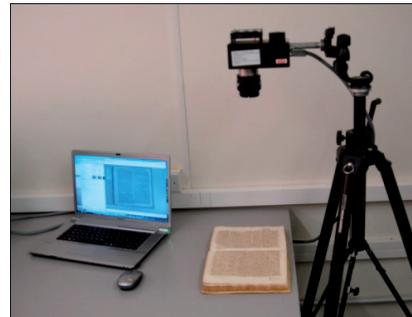
Figure 1: Multispectral imaging set-up.
