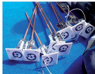
Figure 3: Control point targets
