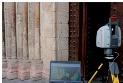
Figure 2: HDS ScanStation 2 during the data acquisition
