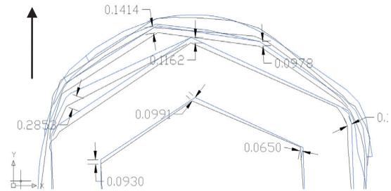
Figure 11: 2D plans from the direct / empirical method (blue line) and laser scanner (black line). For external outline is intended the northern side and for internal the southern one. The measurements indicate the absolute difference comparing the two methods (direct and laser scanner) for some characteristics points of the medieval tower.
