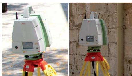
Figure 5: The Laser ScanStation C10 used
