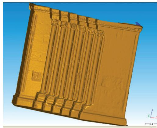
Figure 7: Mesh after cleaning and hole filling
