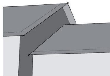
Figure 10: One polyline is above the other: only the overhang of the highest polyline is different to zero.
