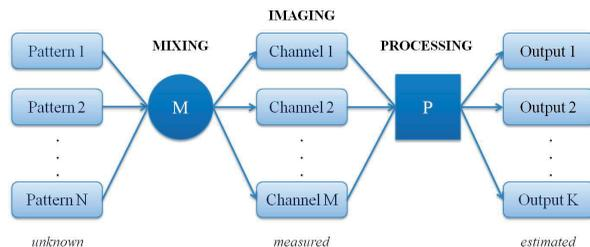
Figure 6: Superposition of different (unknown) patterns in multispectral imaging. Channel selectivity from diversity (measured) images can be translated into pattern selectivity. The outputs are estimates of the patterns.
