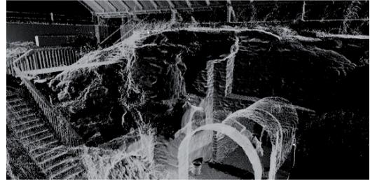
Figure 13: Registration of the point clouds for Saint Theodore in Idalion village. All points clouds are transformed into one coordinate system
