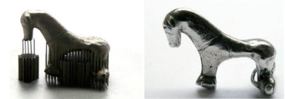
Figure 12: Fibula, Celtic. Selective Laser Melting (SLM). Source: RP-Lab, Aachen University of Applied Sciences, Celtic Museum, Hallein, Austria
