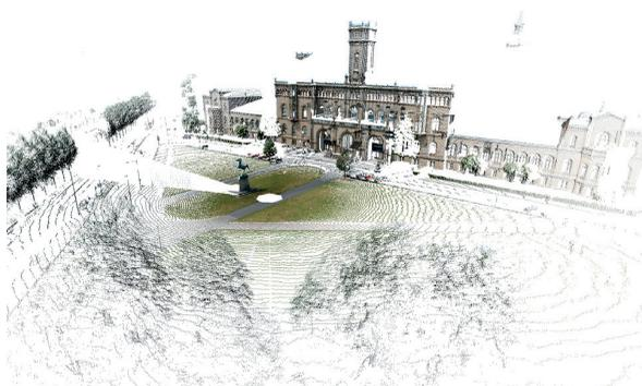
Figure 11: Terrestrial laserscan with texture colors
