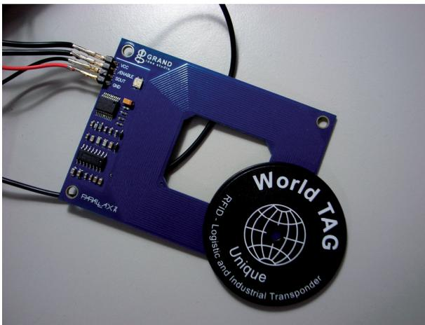
Figure 4: RFID reader and Tags
