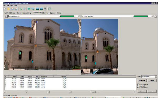
Figure 15: Tie points used in the Hugin software
